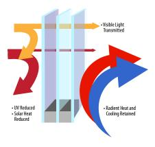
In climates where heating and cooling are the primary concern, HeatSeal Glass products are designed to take advantage of free solar heat, resulting in higher inside glass temperature. Passive solar and thermal insulation reduce the draft sensation caused by cold glass surfaces, providing windows that reduce heating costs.
