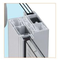
Interlocking meeting rail system with quadruple weather-stripping for controlling infiltration of air, water, dust, and noise. Full length heavy gauge reinforcements in meeting rails and pull rail provide great rigidity and strength.
