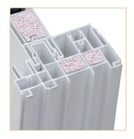
Thermally welded multichambered 5-5/8" main frame provides superior strength and thermal insulation. Optional foam filled insulated extrusions provide better thermal efficiency.
